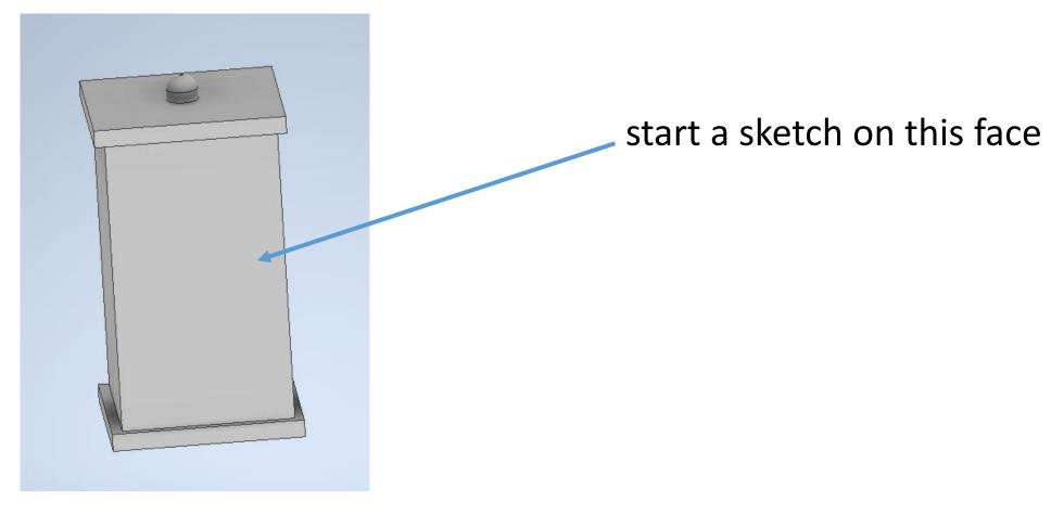
. do this by drawing 2mm strips on each side of the face with a gap of 1.5mm with the edges
