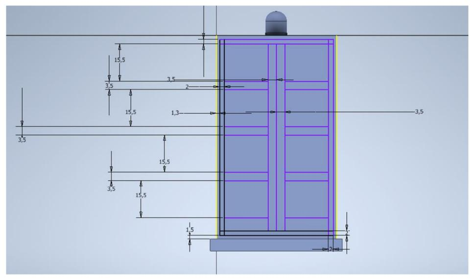
• after finishing this sketch made a 1mm backward extrusion
